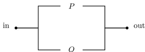
If either  $P$  or  $Q$  is on (T), then the current can flow from the “in” side to the “out” side of the circuit. On the other hand, we can represent  $P \wedge Q$  by a series circuit:
