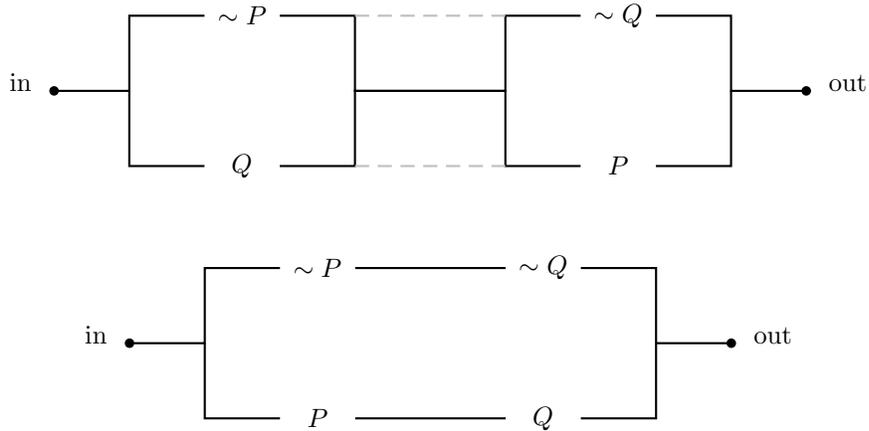
This circuit represents  $[(\sim P) \wedge (\sim Q)] \vee [P \wedge Q]$ , and so we have (as the reader can check)
