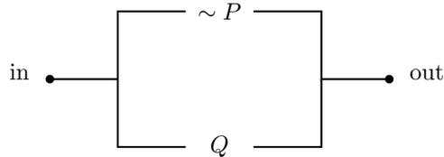
We see that the only time the circuit does *not* flow is when  $P$  is true ( $\sim P$  is false) and  $Q$  is false, so this matches what we know of when  $P \rightarrow Q$  is false. From another perspective, if  $P$  is true, then the top part of the circuit won’t flow so  $Q$  must be true, for the whole circuit to be “on,” or “true.”
