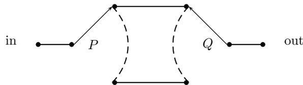
In the above, the switch  $P$  is in the “up” position when  $P$  is ‘true, and “down” when  $P$  is false. Similarly with  $Q$ .
